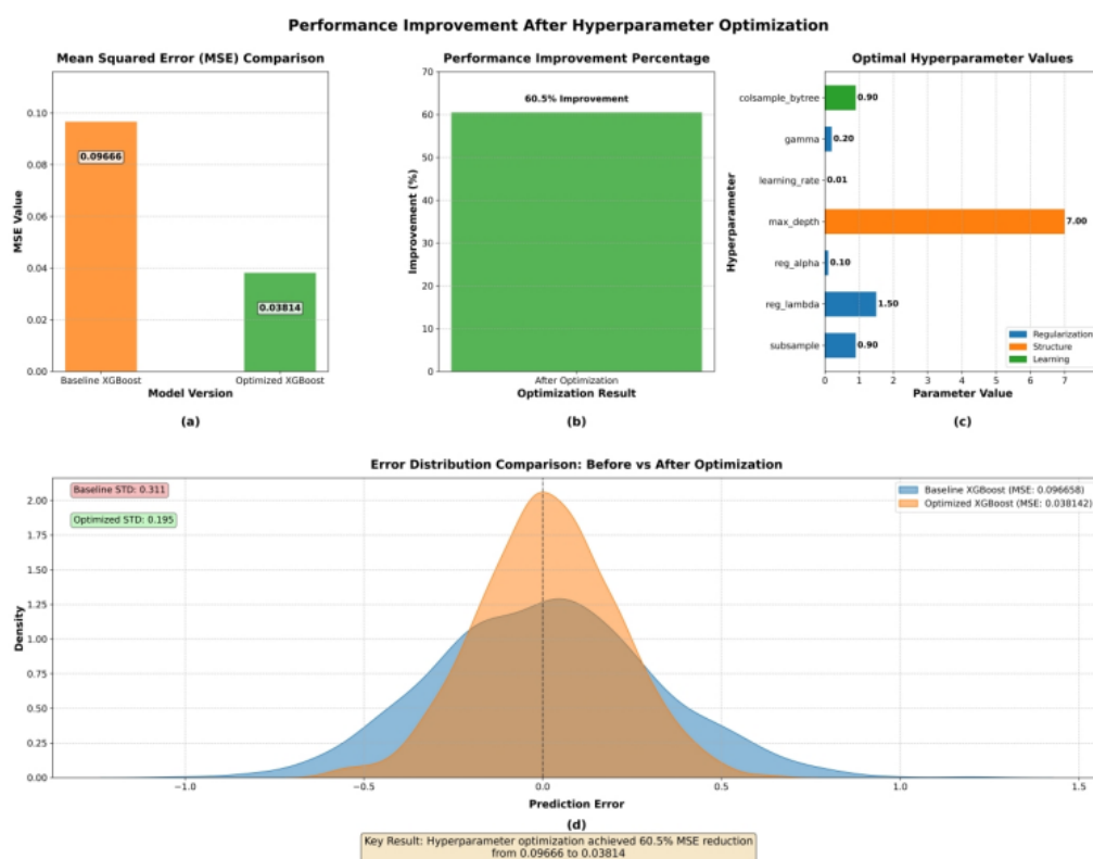
Figure 3. Hyperparameter optimization results (photo/picture credit: original)
